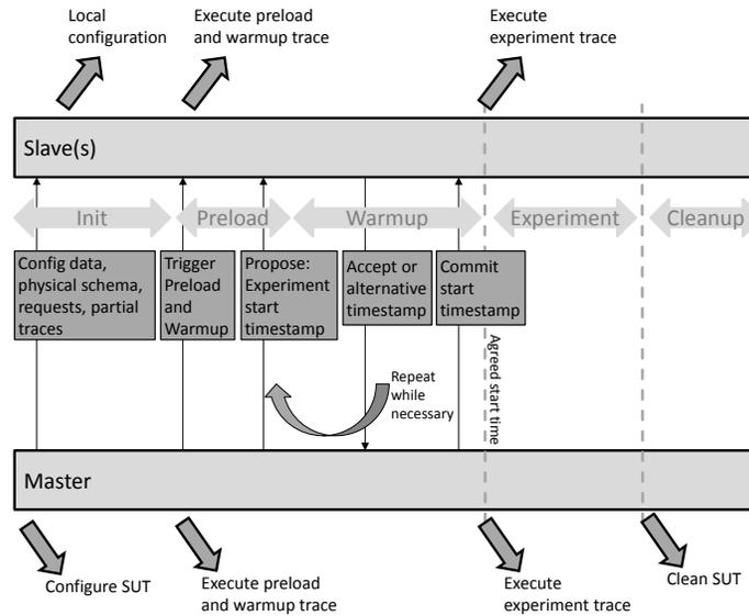
Fig. 2: Execution Phases and Distributed Coordination
